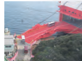
Wheeled vehicles are directly driven on and off as on a ferry
