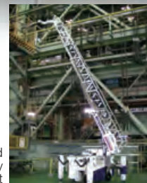
Valve opening and closing operated by remote-controlled robot
