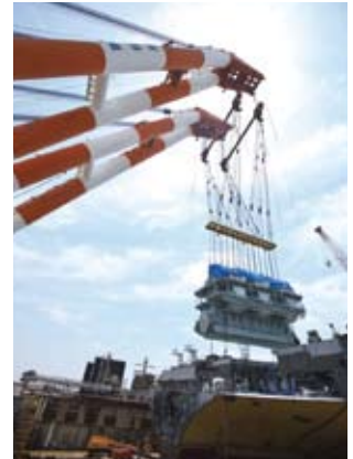
A giant crane installing an engine into place
