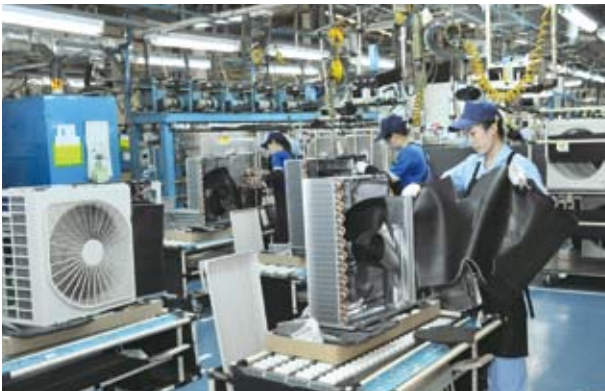
Assembling air-conditioner outdoor units
