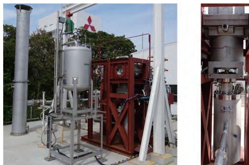
Figure 35 Liquid hydrogen pressure booster pump for hydrogen fueling stations
